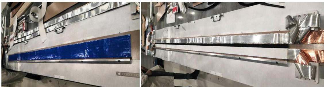
Fig. 19. Lay up of the glue film (left), and the Flexible Conductor Cable underneath.
