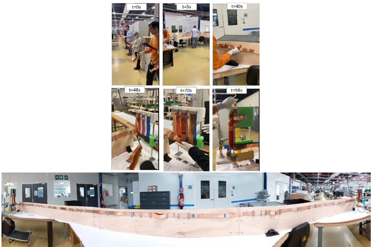
Fig. 16. Harness integration test (above) and final result on a 9 m long internal inter-tank mockup (below).
