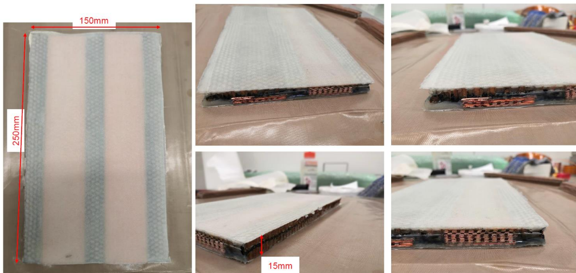
Fig. 11. Composite derisk mockup for external raceway harness.
