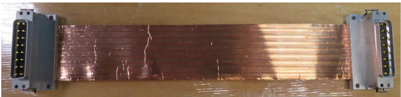
Fig. 14. Mating of the FCC with the connectors.
