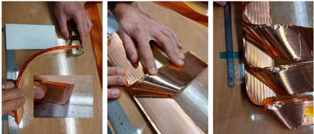
Fig. 8. Mock-up derisk on internal inter-tank harness.
